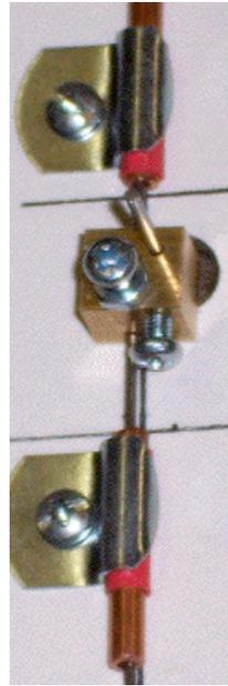
4. The Point-wit, control wire and tubes are arranged as shown. A short length of tube is used on one side to support the control wire. On the other side, the tube continues to the Lever Frame. The tubes are clamped clear of the 8mm and 15mm marks and in line with the 3mm offset line.
