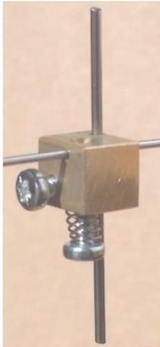
The vertical rod is set to engage with the tie rod of the points and is fixed in position by the horizontal screw. The other screw (sprung) adjusts the pressure on a clutch which grips the control wire as it passes through Point-wit. The pressure is set such that there is sufficient grip to operate
