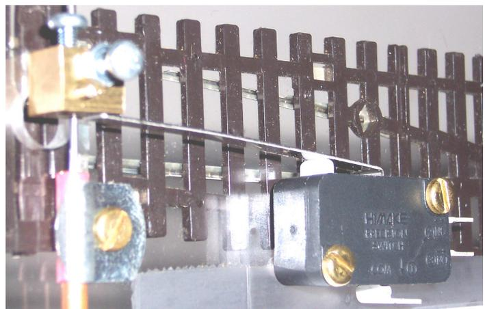
**Timing is important.** It is important that the switch changes state while the point blades are in the middle of their stroke. If the switch changes while the blades are still in contact with one of the running rails, then a short circuit will exist. This is particularly critical with DCC operation. The timing can be adjusted by gently flexing the switch's lever. It's designed with that in mind. You will hear the switch click at the changeover.
