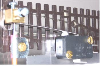
flexing the switch's lever. It's designed with that in mind. You will hear the switch click at the changeover.
