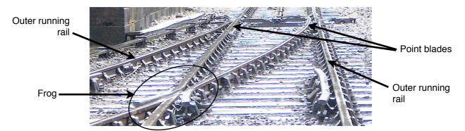
pointwork. However, they also complicate wiring. A live frog turnout comprises three electrical elements. Two are the outer running rails. The third is everything else - the frog and the rails connected to it, as well as the point blades. As the points change, the frog becomes electrically connected to one or other of the outer running rails according to which one the blades touch. The *polarity* of the frog is said to change.
